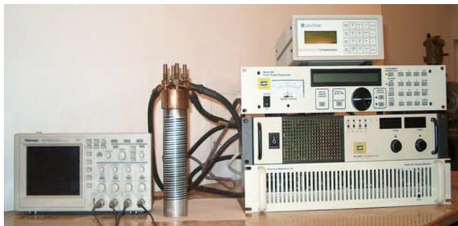
Fig. 11. Experimental system (resistive-type SFCL shown without cryostat).
