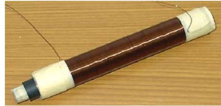
Fig. 8. Model of 1210 A superconducting fault current limiter with open magnetic core.
