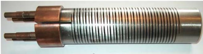
Fig. 10. Bi-2212 bifilar coil (C02-034 bifilar coil made by Nexans)
