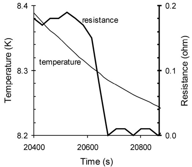
Fig. 5. Temperature and resistance during superconducting transition of the NbTi magnet.
