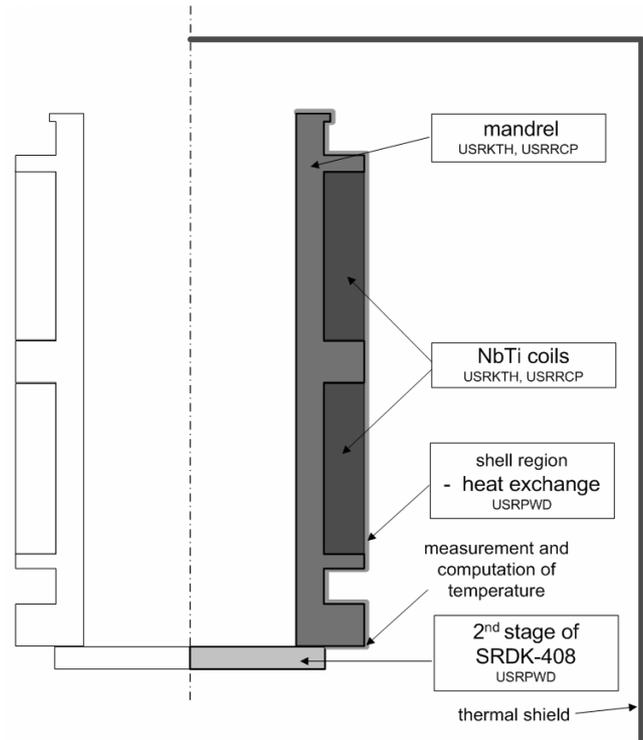
Fig. 8. Geometry of numerical model in FLUX2D.
