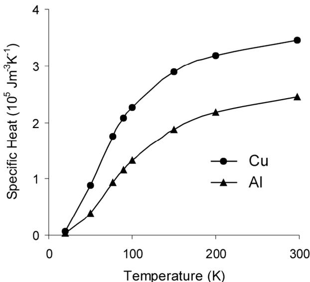
Fig. 7. Specific heat vs. temperature for Cu and Al.
