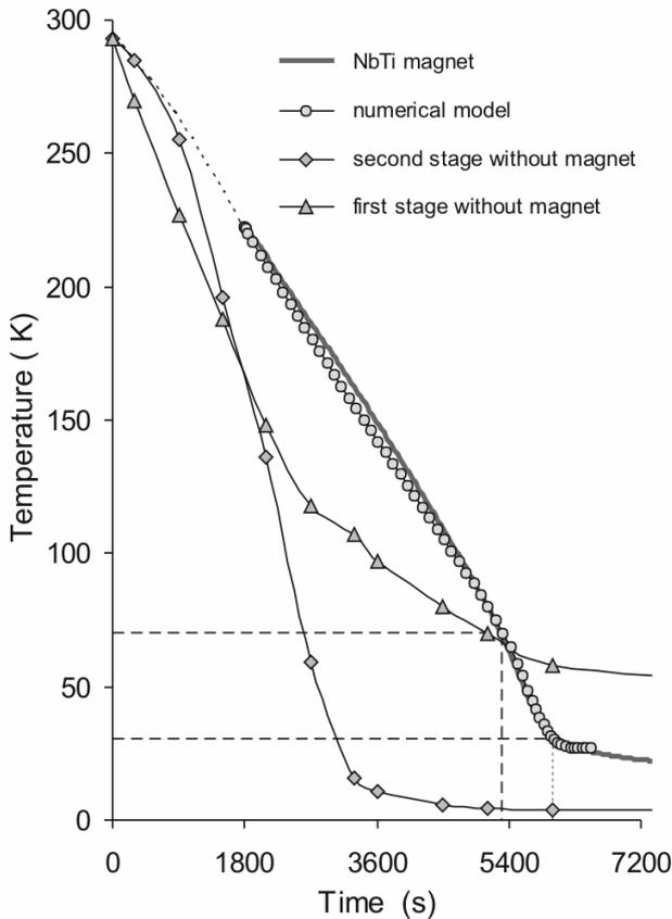
Fig. 9. Temperature of the first and the second stage of SRDK-408 without magnet and temperature of NbTi magnet.
