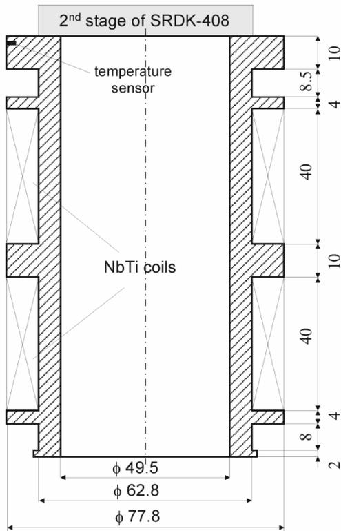
Fig. 3. AL-alloy mandrel of the NbTi magnet. Dimensions in mm.
