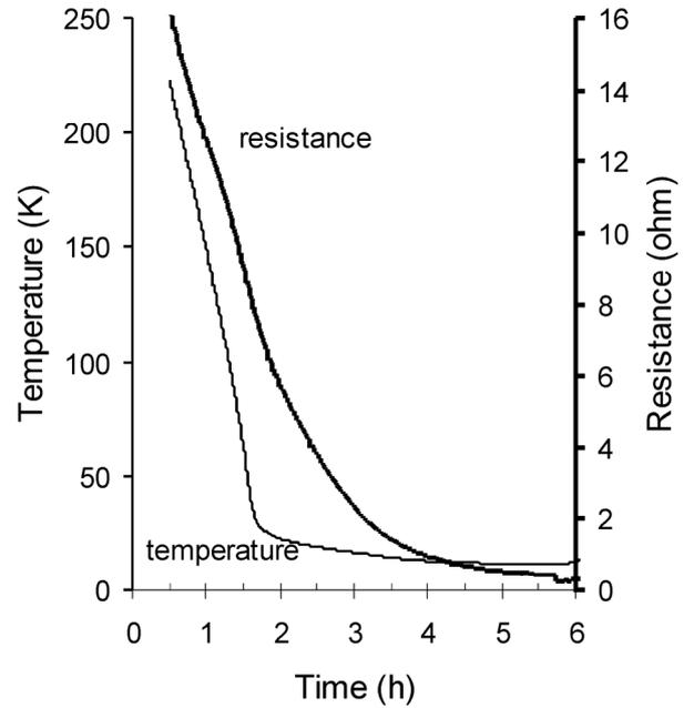
Fig. 4. Temperature and resistance during cooling down of the NbTi magnet.
