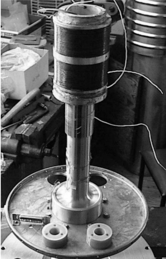
Fig. 2. NbTi magnet connected to the second stage and top part of the thermal shield connected to the first stage of SRDK-408 cryocooler.
