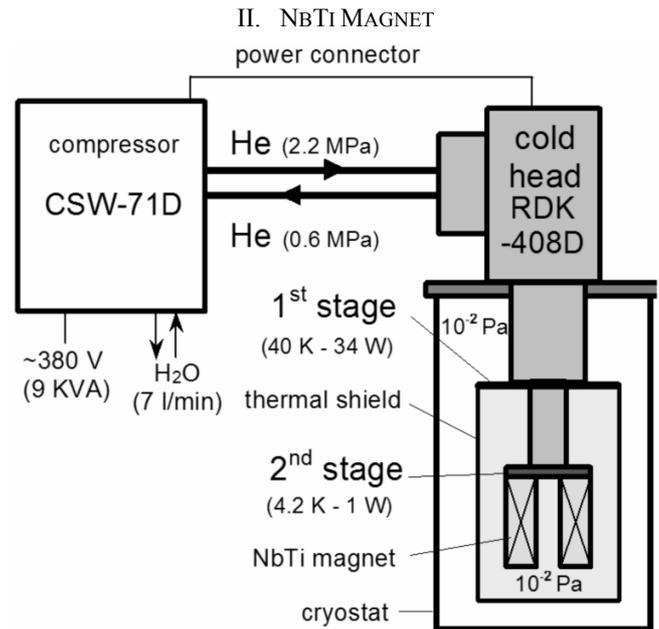
Fig. 1. The NbTi magnet with a cooling system using the SRDK-408 cryocooler.
