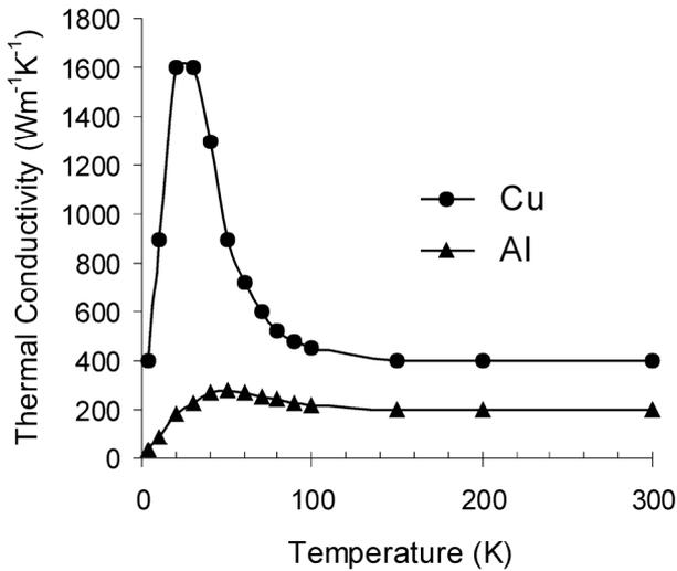
Fig. 6. Thermal conductivity vs. temperature for Cu and Al.
