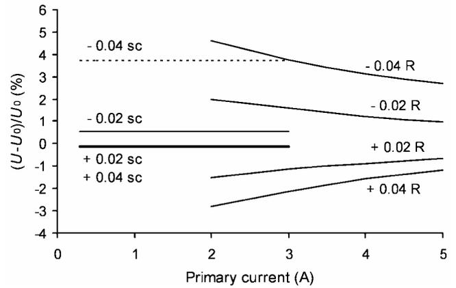
Fig. 6. Changes in  $V-I$  characteristics vs the height of window of iron core in resistive (R) and superconducting (sc) state at 77 K.
