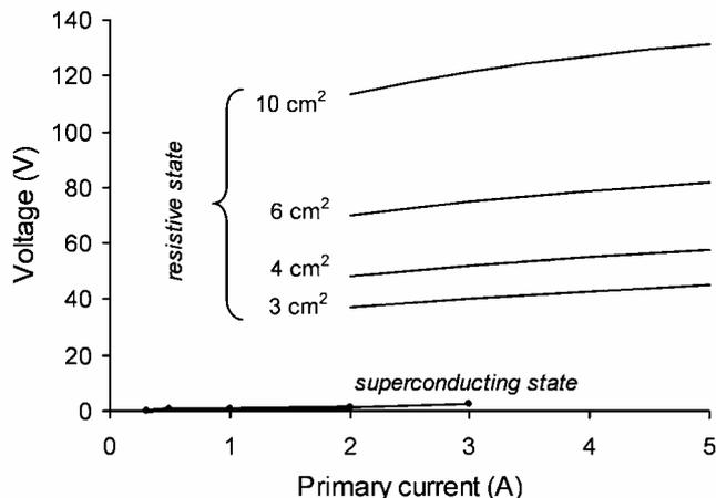
Fig. 8. Changes in resistive and superconducting state  $V-I$  characteristics of numerical model of inductive SFCL at 77 K vs the cross-section of iron core.
