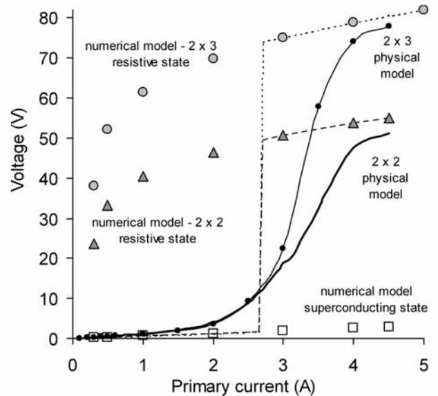
Fig. 4.  $V-I$  characteristics of physical models with 2 cm x 2 cm and 2 cm x 3 cm iron core cross-sections and respective numerical model characteristics in superconducting state and resistive state at 77 K.
