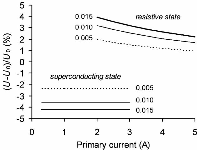
Fig. 5. Changes in  $V-I$  characteristics vs the breadth of window of iron core in resistive state and superconducting state at 77 K.
