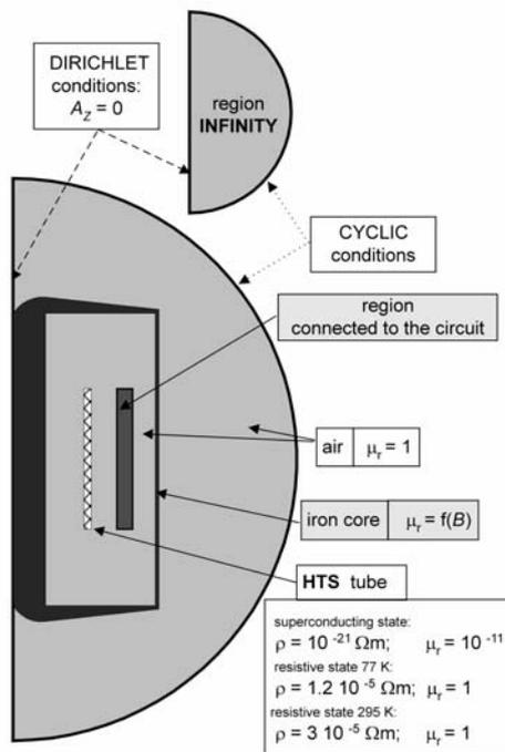
Fig. 2. Geometry and region properties diagram in FEM part of numerical model of inductive SFCL – FLUX2D.
