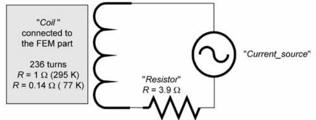
Fig. 3. Diagram of circuit part of numerical model of inductive SFCL – FLUX2D.
