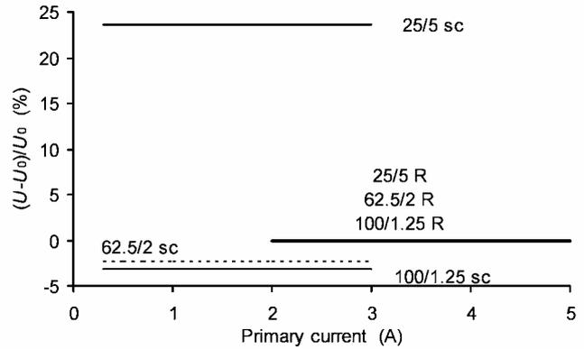
Fig. 7. Changes in resistive (R) and superconducting (sc) state  $V-I$  characteristics of numerical model vs the shape of superconducting tube (height (mm)/thickness (mm)) at 77 K.
