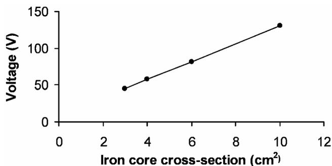
Fig. 9. Voltage drop on inductive SFCL vs iron core cross-section area for current = 5 A at 77 K.
