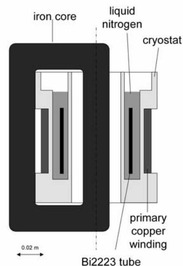
Fig. 1 Inductive superconducting fault current limiter.
