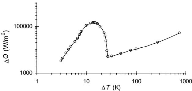
Fig. 3. Heat transfer  $\Delta Q$  from a metal surface to  $IN_2$  at 77 K vs.  $\Delta T$  between surface and  $IN_2$  under normal atmospheric pressure [2], [1].
