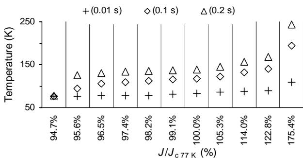
Fig. 10. Maximum temperature for different  $J/J_{c77K}$  and time.
