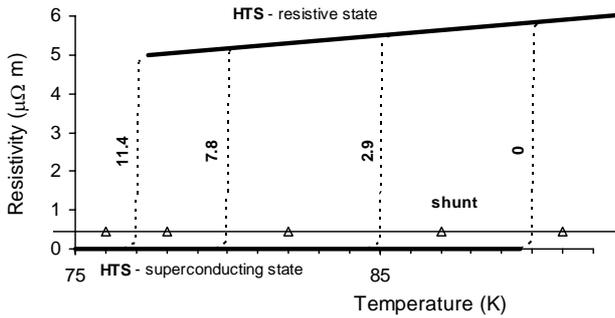
Fig. 2. Resistivity of shunt and HTS [1] vs. temperature for different current density ( $A/mm^2$ ).
