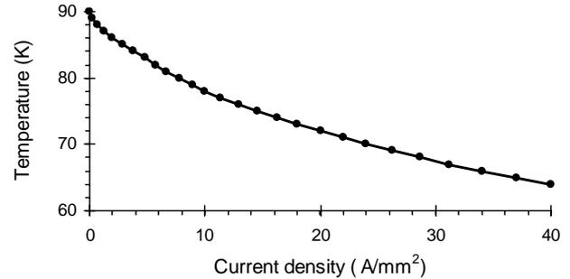
Fig. 5. Critical temperature of Bi-2212 bifilar coil vs. current density (self magnetic field) [7]-[9], [1].
