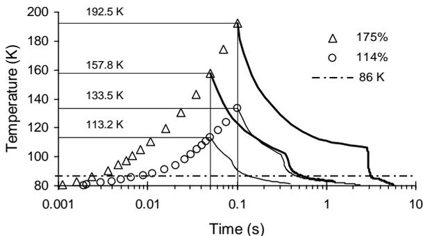
Fig. 11. Temperature vs. time for different  $J/J_{c77K}$  and for different time to switch off the current by breaker.
