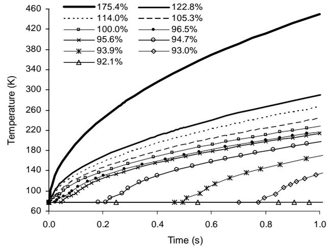
Fig. 6. Maximum temperature in limiter vs. time for different  $J/J_{c77K}$ .
