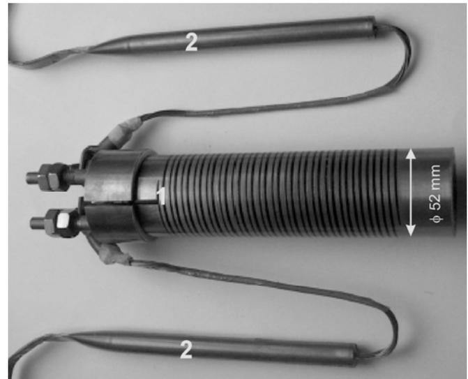
Fig. 1. Superconducting elements of resistive SFCL:
