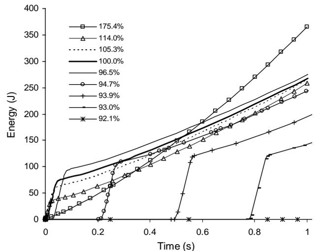
Fig. 8. Energy transferred to  $IN_2$  vs. time for different  $J/J_{c77K}$ .
