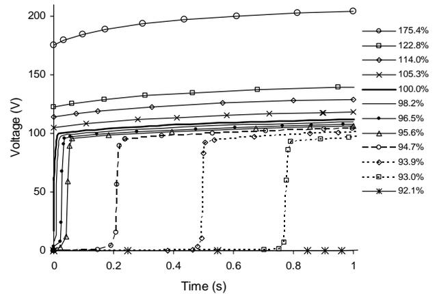
Fig. 7. Voltage in limiter vs. time for different  $J/J_{c77K}$ .
