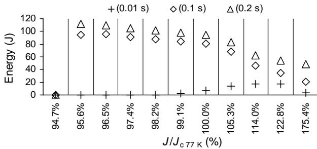
Fig. 9. Energy transferred to  $\text{LN}_2$  for different  $J/J_{c77K}$  and time.
