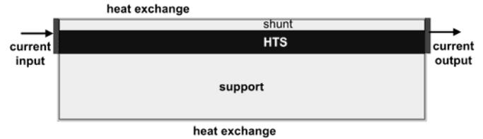
Fig. 4. Simplified geometry of FEM numerical model of resistive SFCL in electro-thermal application of FLUX2D [1].
